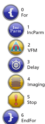
Figure 3. MacroBuilder scripts are simply created using drag-and-drop modules. Here, a single loop was set to repeat 190 times, collecting MFM images after incrementing the field strength by 5 G at each step.
