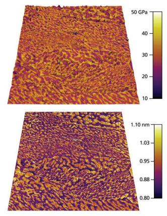
(top) Storage modulus and (bottom) indentation depth overlaid on topography for tin/lead alloy solder. Tin-rich (yellow) and lead-rich (purple) regions can be identified in the storage modulus map. Scan size 23 µm. Images acquired on a Cypher S AFM at 2 Hz scan rate with blueDrive photothermal excitation.
