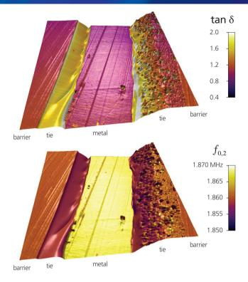
(top) Loss tangent and (bottom) frequency for a commercial coffee packaging bag in cross section. Both images distinguish between the different sample components (vapor barriers, "tie" layers, and metal layer). Scan size 15 µm. Acquired with a Cypher S.
