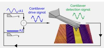
**Figure 1**: Schematic representation of AM-FM imaging of multilayer polymer film composed of from left to right: polyethylene terephthalate (PET), polyethylene (PE), ethyl vinyl alcohol (EVOH), PE and polypropylene (PP).
