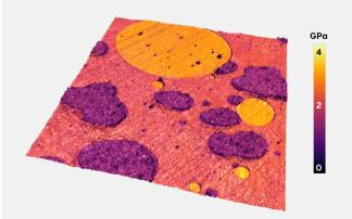
**Figure 2:** Polymer blend sample composed of polyethylene (darkest), polypropylene (matrix) and polystyrene (brightest). The 3D overlay of elastic modulus on topography. Image size: 25 um.
