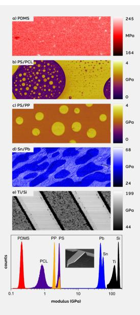
**Figure 5:** AM-FM modulus images of a) PDMS, b) PS/PCL polymer blend, c) PS/PP polymer blend, d) Sn/Pb solder alloy, and e) Ti thin-film stripes on Si. Bottom: Combined histogram of all the images using the same type of cantilever. The inset shows a scanning electron micrograph of an Olympus AC160 cantilever that was used in all these measurements.
