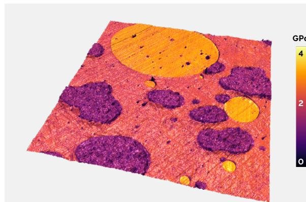
Figure 2: Polymer blend sample composed of polyethylene (darkest), polypropylene (matrix) and polystyrene (brightest). The 3D overlay of elastic modulus on topography. Image size: 25  $\mu\text{m}$ .
