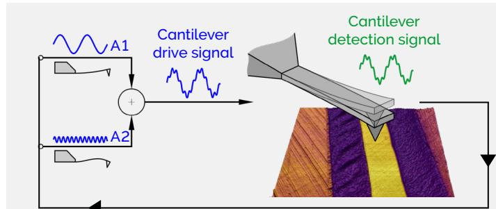
Figure 1: Schematic representation of AM-FM imaging of multilayer polymer film composed from left to right: polyethylene terephthalate (PET), polyethylene (PE), ethyl vinyl alcohol (EVOH), PE and polypropylene (PP).
