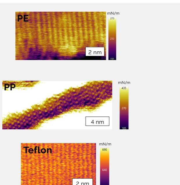
Figure 3: Molecular level tip-sample stiffness images of polyethylene (PE) chains, polypropylene (PP) and Teflon.
