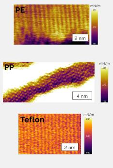
Figure 3: Molecular level tip-sample stiffness images of polyethylene (PE) chains, polypropylene (PP) and Teflon.
