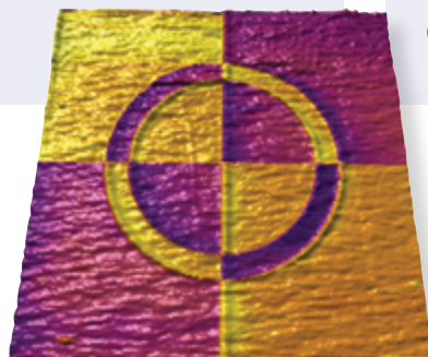
PFM of BTO thin film Piezoresponse Force Microscopy (PFM) phase image of an 8 nm thick BTO layer grown on a GaAs / \text{Al}_{0.3}\text{Ga}_{0.7}\text{As} heterojunction to make confined quantum wells. The sample was poled with a DC bias to create the pattern shown, 10 \mu\text{m} scan. Image courtesy of F. Bi and G. Jnawali, Levy Research Group, University of Pittsburgh.
