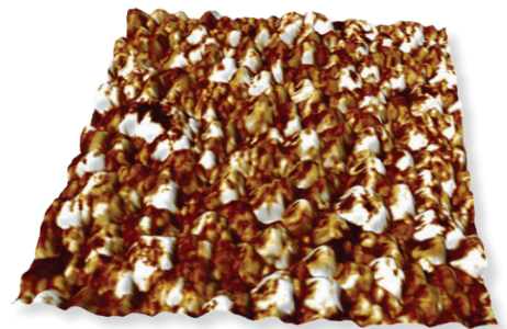
CAFM image of Europium-doped ZnO sample, 2 \mu\text{m} scan. Sample courtesy of the Krishnan Lab, Univ. of Washington.
