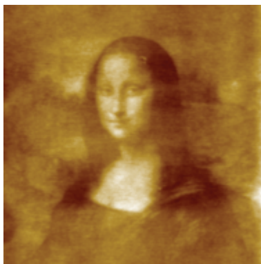
Nanolithography example created by anodic oxidation on silicon, 20 µm scan.
