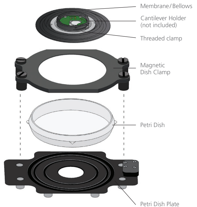
Schematic of the Petri Dish Heater assembly (top). The Heater plate easily fits on the MFP-3D scanner (bottom photo).
